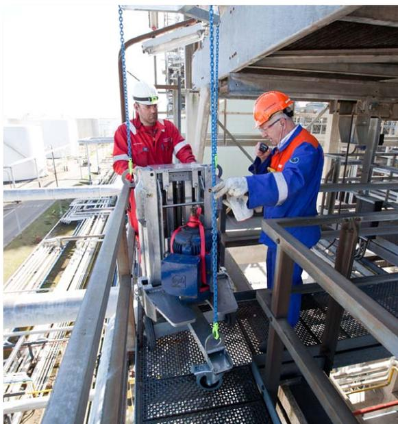
The lifter is also provided with two forklift pockets to allow the machine to be shifted easily. The lifter has been tested and is provided with a TÜV test certificate. Once the electric motor is placed on the lifter, the lifter can only be shifted if it is in its lowest position. **The lifter may not be rolled away with the electric motor on board at any other height.**
